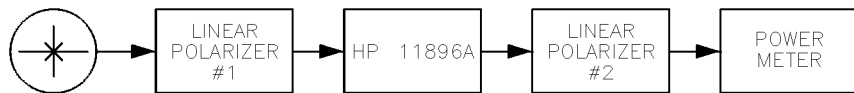
Figure B-1. Block diagram for testing the extinction ratio of the HP 11896A.
